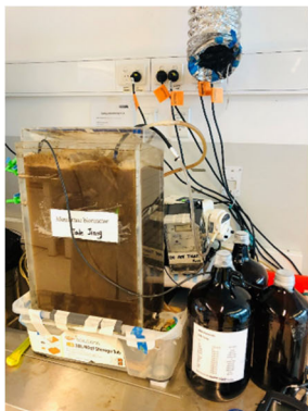
Lab-scale MBR reactor (20 L)
