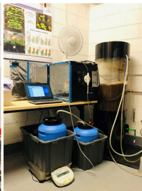
Pilot-scale MBR reactor (100 L)
